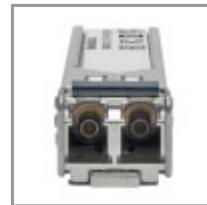
Adds an LC female connector to your HP 10/100/1000 network equipment.
