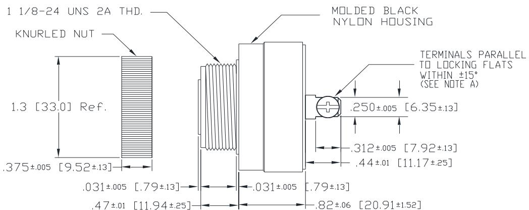
NOTE A: TERMINALS-.032 BRASS TIN PLATED, TAPPED FOR #6-32 SCREW. TWO #6-32 NICKEL PLATED BRASS SCREWS INCLUDED. WILL ACCEPT 1/4" QUICK CONNECT.
