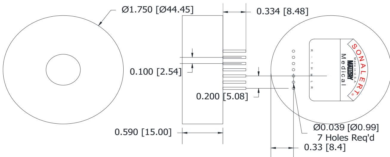
**NOTE:** Alarm functions at max dB. If a lower sound output is desired, add a 1/4 W resistor valued from 27k $\Omega$  down to a minimum 100 $\Omega$  to achieve the desired sound level output. PIN OUT is R - + H M L R.
