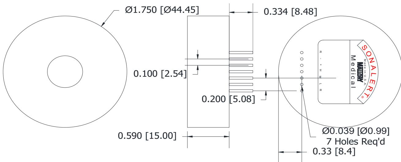
**NOTE:** Alarm functions at max dB. If a lower sound output is desired, add a 1/4 W resistor valued from 27kΩ down to a minimum 100Ω to achieve the desired sound level output. PIN OUT is R - + H M L R.
