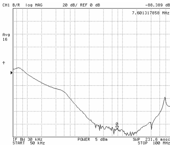
Figure 3 - Common Mode attenuation, 0.05-100 MHz. Source and load resistances are 50 Ω. Two 0.1 μF Y-caps to common line. Vertical scale: 20 dB/div, with zero dB level marked by arrow.
