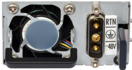
Figure 9. Input polarity marking
