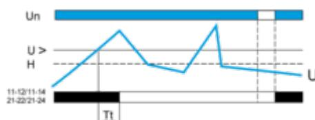
**Legend****Tt** Time delay after crossing of threshold**Un** Nominal supply voltage**U** Monitored supply voltage**H** Hysteresis**U>** Overvoltage threshold**U<** Undervoltage threshold
