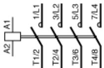
3-Pole Contactors: 3P + N/C
