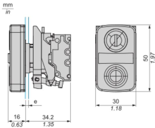
e : Clamping thickness: 1 to 6 mm / 0.04 to 0.24 in.
