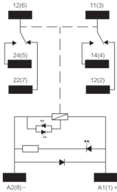
**NOTE:** For DC input , A1 have to be + , otherwise it would short circuit from protection module
