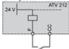
“PLC” position with PLC transistor outputs
