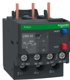
Thermal overload relay, TeSys Deca, 23-32A, 1NO+1NC, class 10A, lugs ring terminal
