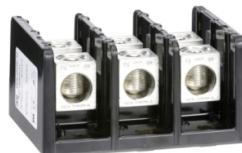
Power distribution block, Linergy, 3 pole, 1 line, 1 load, 310A Cu, 250A Al, 600V
