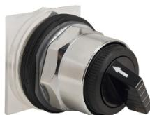
Selector switch head, Harmony 9001K, metal, standard handle, black, 30mm, 2 positions, Cam D, stay put
