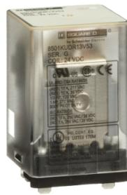
Plug in relay, Type KU, blade, 0.5 HP at 240 VAC, 10A resistive at 120 VAC, 11 blade, 3PDT, 3 NO, 3 NC, 24 VDC coil
