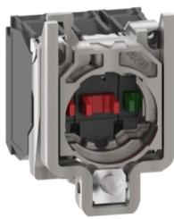
Complete body contact assembly, Harmony XB4, for push buttons or selector switches, single contact block with body fixing collar 1NC faston connector
