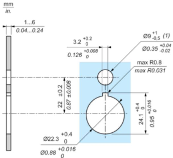
(1) : For IP X9 applications, the max recommendation dimension of hole is Ø9 mm/Ø0.35 in.
