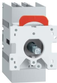
Disconnect switch, TeSys VLS, body switch, 16A, 10HP at 480VAC, UL508, three phase, 5kA SCCR, size 1, door mount
