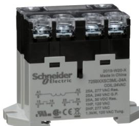
**Power relay, SE Relays, 25A, 2NO, 24VAC, LED push button, screw terminals, DIN or panel mount**
