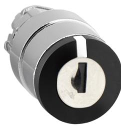
Key switch selector head, Harmony XB4, metal, black, 22mm, key 455, 3 positions, spring return from right to center, key withdrawal left and center
