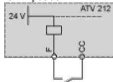
“PLC” position with PLC transistor outputs
