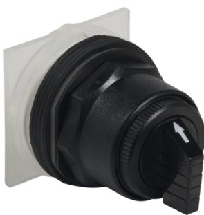
Head for selector switch, Harmony 9001SK, plastic, standard handle, black, 30mm, 3 positions, return both sides to center, cam code 2
