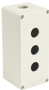
22mm push button, Harmony XALD, empty grey enclosure, die cast zinc alloy, 3 openings, vertical mount, NEMA 4, 13
