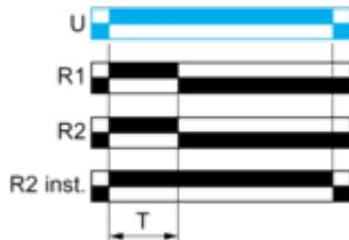
**Function Hw: Interval Relay & with Retrigger / Restart Control****Description**
