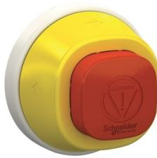
Illuminated emergency stop head, Harmony XB5, plastic, red, 22mm, trigger latching turn to release, red LED, 230...240V AC
