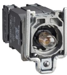
Complete body/contact assembly and light block, Harmony XB4, with body/fixing collar, BA9s incandescent bulb, 110...120V, 1NO + 1NC
