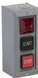
Push button, Type B, standard duty control station, 5A, 600 VAC, START/STOP, red pilot light, NEMA 1
