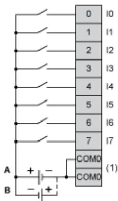
(1) The COM0 terminals are connected internally.
