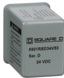
Plug in relay, Type R, hermetically sealed miniature, 5A resistive at 240 VAC, 14 blade, 4PDT, 4 NO, 4 NC, 24 VDC coil
