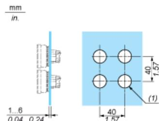
(1) Ø22.5 mm recommended ( $\varnothing 22.3_0^{+0.4}$ ) / Ø0.89 in. recommended ( $\varnothing 0.88_0^{+0.016}$ )
