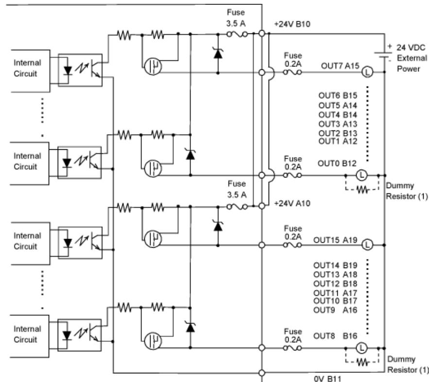
(1) (Example) The output delay time (OFF to ON) is 1.5  $\mu$ s where the output current is 50 mA. Install an external dummy resistor to increase the amount of current when faster response is required when the load is light.
