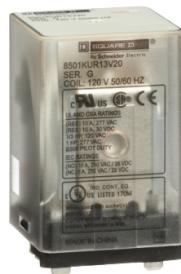
Relay, Harmony 8501K, 3PDT, 11 blades, coil, 10A resistive at 120V AC, 0.5 HP at 240V AC, 120V AC, 3NO + 3NC
