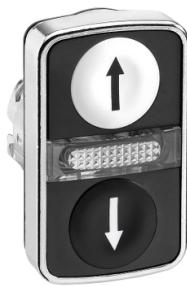
Illuminated double headed push button head, Harmony XB4, metal, 22mm, 1 white flush UP ARROW + 1 pilot light + 1 black flush DOWN ARROW
