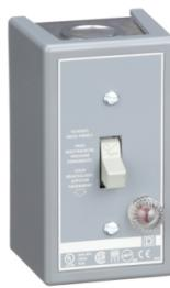
Manual Starter, fractional horsepower, 16A, 1 pole, 1 HP at 277 VAC, toggle operated, red indicator, NEMA 1 enclosure
