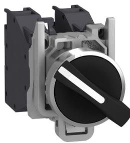
Selector switch, Harmony XB4 - ATEX D, metal, 22mm, 2 positions, black standard handle, stay put, screw clamp terminals, 1NO + 1NC
