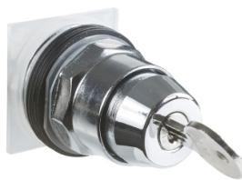
Selector switch, Harmony 9001K, metal, key switch, key active left, 30mm, key E10, 2 positions, Cam E, stay put, 1 CO
