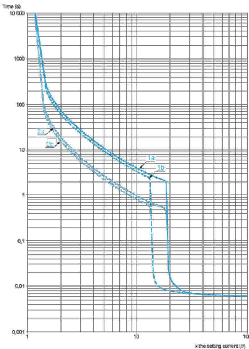
1a 3 poles from cold state ( $I_r$  minimum): GV3P1b 3 poles from cold state ( $I_r$  maximum): GV3P2a 3 poles from hot state ( $I_r$  minimum): GV3P2b 3 poles from hot state ( $I_r$  maximum): GV3P
