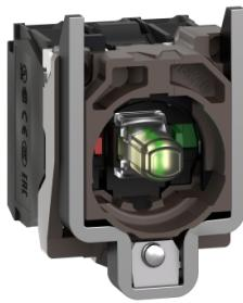
Complete body contact assembly and light block, Harmony XB4, metal, universal LED, body fixing collar, 1NO + 1NC, 110...120V AC
