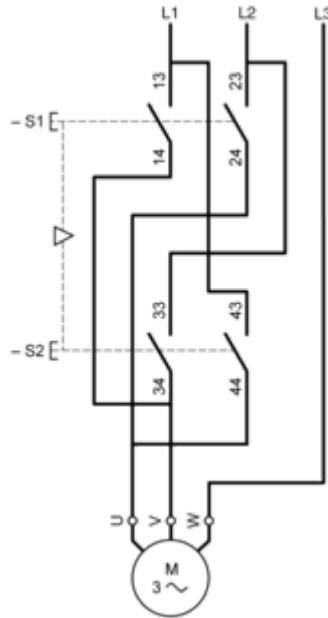
Combined with 3-pole isolating block XACS399 or XACS3991, shown in the unoperated position (pendant station "supplied"), fitted with key release trigger action latching Emergency stop operator.
