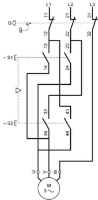
**Control of 2-Speed Reversing Motor 2-Phase Switching**
