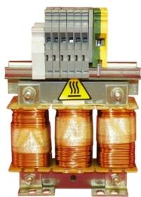
line/motor choke - 0.5 mH - 60 A - 3 phases - 94 W - for variable speed drive
