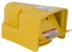
Foot Switch, Harmony 9002AW, industrial, oversized pedal and side shields, DPDT contact, with safety door, 10A at 600V AC
