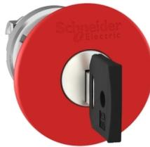
Head for emergency switching off push button, Harmony XB4, red 40mm stop, 22mm trigger and latching key release, key 421E
