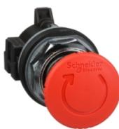
Emergency stop head, Harmony 9001K, switching off, metal, red mushroom 40mm, 30 mm, trigger latching turn to release
