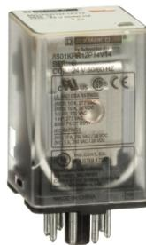
Plug in relay, Type KP, tubular, 1 HP at 277 VAC, 10A resistive at 120 VAC, DPDT, 2 NO, 2 NC, 24 VAC coil, pilot light
