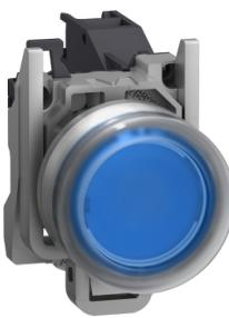
Complete push button, Harmony XB4 - ATEX D, blue projecting with boot, metal, 22mm, spring return, 1NO, for insertion of legend
