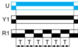
**Function: 2 Output with Retrigger / Restart Control**
