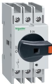
Disconnect switch, TeSys VLS, body switch, 16A, 10HP at 480VAC, UL508, three phase, 5kA SCCR, size 1, DIN rail mount
