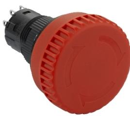
Complete illuminated mushroom head push button, Harmony XB6E, 16mm, red pushbutton, 32mm, trigger turn pull to release, 2NC
