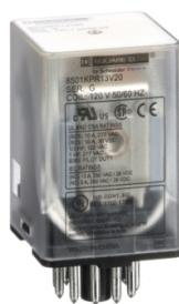
Plug in relay, Type KP, tubular, 1 HP at 277 VAC, 10A resistive at 120 VAC, 11 pin, 3PDT, 3 NO, 3 NC, 120 VAC coil
