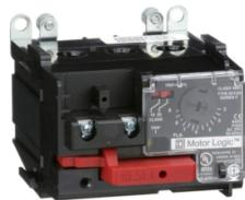
Overload Relay, Motor Logic, solid state overload relay, NEMA Size 00, 3 pole, 3A to 9A, 600VAC, separate mount
